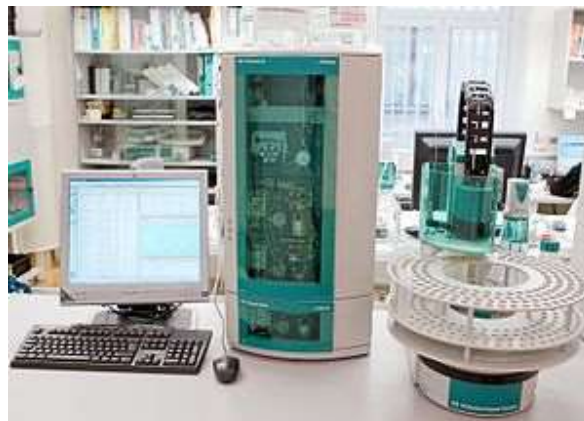
Metrohm 850 Ion chromatography system
